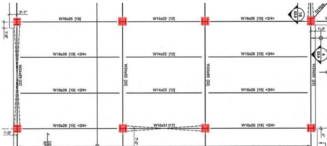
Figure 5: Typical column layout
